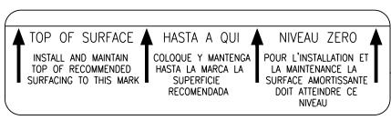
The sticker shown above has been provided to assist with the maintenance of your ground cover. After installing the ground cover, these stickers should be placed on the post by the installer (as shown). Peel the backing away from the sticker and attach it to the post so that the line is level with the top of your ground cover. As erosion or compaction of surfacing occurs, the line will be visible. This will indicate that it is time to add material to your surfacing.
